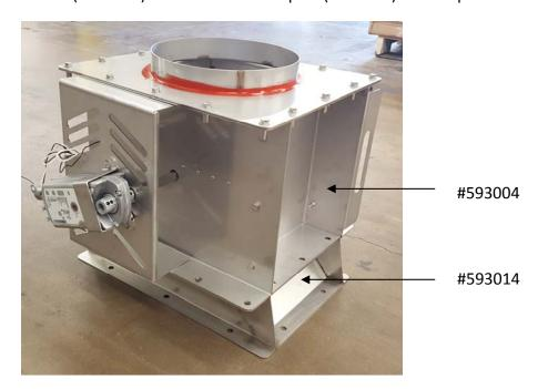
Actions Required (continued): The single damper smoke extractor is 2 1/4" (57mm) taller than the dual damper smoke extractor and the adapter is 4" (102mm) tall, this will require some adjustment to the length of the exhaust duct. The actuator motor of the single damper smoke extractor does not have a port for the conduit connection for the smoke extractor exhaust fan; some modification will be required.
