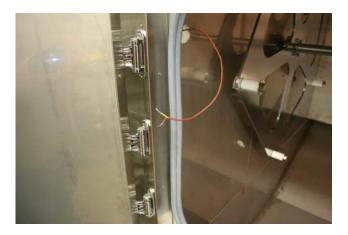
4. Cut the new thermocouple wires about 3 inches back from the thermocouple mounting plate. Strip the ends of the thermocouple wires. The stripped portion of the wire should not be more than 1/4" and should not be exposed once the splice is placed on the wire.
