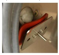
2. Cut the wires from the old thermocouple approximately 3 inches from the back of the thermocouple mounting plate.
